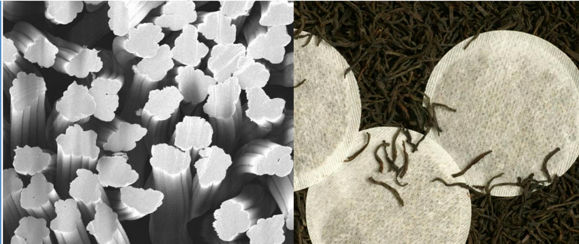
Our short cut fibres with cut lengths of 3 to 12 mm deliver perfect dispersion in all wet-laid processes for the production of paper or nonwovens. The paper porosity can be precisely controlled by incorporating viscose fibre, while our other speciality fibres can help increase the tear resistance of the paper without loss of tear strength. Viscose fibres are 100% cellulosic and can therefore be easily incorporated into the paper matrix.
