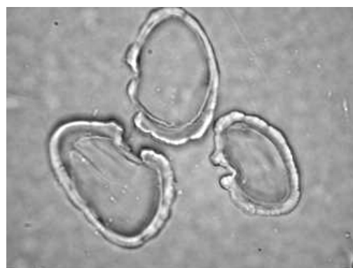
Cross-section of wet Bramante fibre
